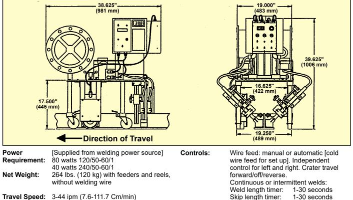
Travel Speed:3-44 ipm (7.6-111.7 Cm/min)<br/>[Digital carriage speed readout- ipm or cm/min]
